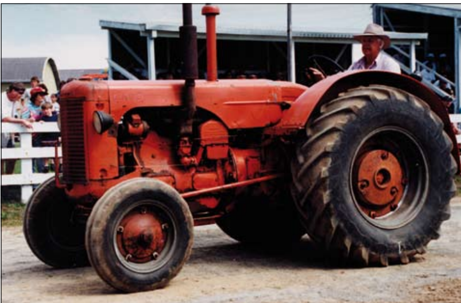
An LA Case in its working clothes, owned by Gus Raymond, attracting much interest from spectators at The 2004 Rusty Iron Rally. Note the oil bath air cleaner reservoir, to the rear of the exhaust pipe. Adjacent, is the hot box which pre-heats the kerosene. (Photo IMJ)
