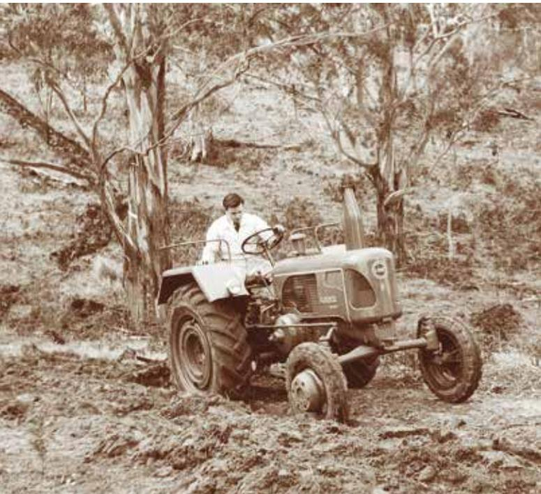
**I demonstrate the Model H to a farmer at Porters Retreat, before the tractor was transported to Orange. Despite being rated at 24 hp, owing to the amazing torque characteristics of the single cylinder two stroke semi diesel engine, its draw bar pull exceeded that of any other tractor rated up to 50 hp.**
